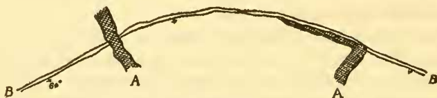
FIG. 2.—SHOWING RELATION OF DIKES (A) TO VEIN (B) ON NO. 1 LEVEL OF MARSH MINE.
